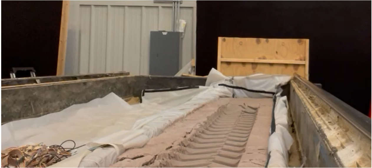
Figure 4.4: RGB view of a test terrain with artificial obstacles: The image shows a controlled experimental setup featuring a terrain with visible tracks, simulating real-world conditions for testing terrain segmentation and obstacle detection systems
