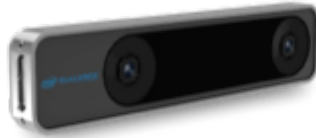
Figure 4.2: Intel RealSense T265 tracking camera provides 6DoF pose and inertial information through visual-inertial odometry (VIO), enabling robust localization in GNSS-denied environments.
