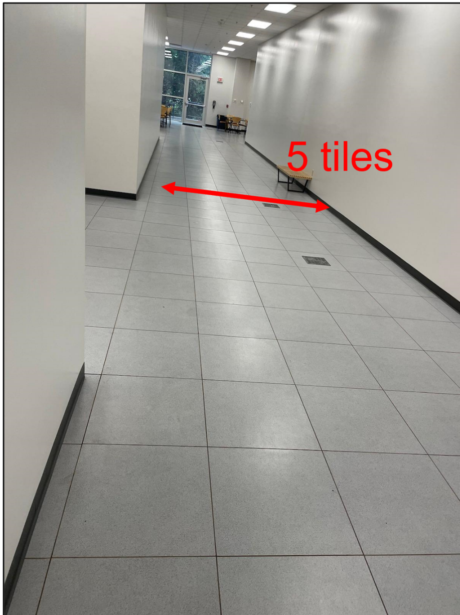
Figure 4.13: Validation of 2D occupancy grid mapping in an indoor hallway environment. Top: Photograph of the hallway with tiled floors (each tile 60\text{ cm} \times 60\text{ cm} ), showing a distance of 5 tiles (3 m) between walls
