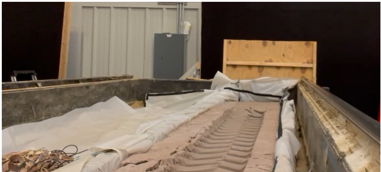
Figure 4.16: Terramechanics rig: Controlled experimental facility with visible terrain features in the order of centimeters. The experimental rig consists of a carriage that allows for longitudinal motion along the rut, which was used for testing the accuracy of the on-board navigation system
